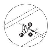
Step 2: Example of fixing the fittings on the wall.
